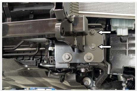
38. Secure the outside of the winch mount using four (two each side) M12 x 1.75 x 40mm hex bolts, eight M12 x 24mm flat washers, four M12 spring washers and four M12 hex nuts. Finger tighten only.
