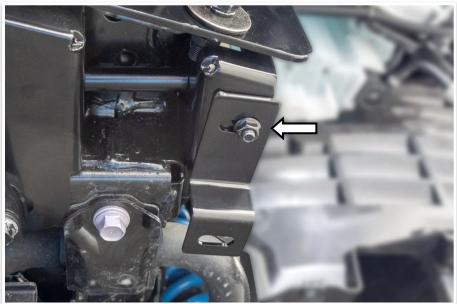
81. Fit the outer bash plate support brackets (item # 12) using M8 combo bolts and M8 flange nuts.
