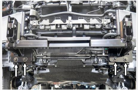
37. Lift the winch frame (item# 2) into position. Secure to the chassis end plates using four M12 x 1.25 x 35mm hex bolts, M12 spring and flat washers. Leave finger tight.
