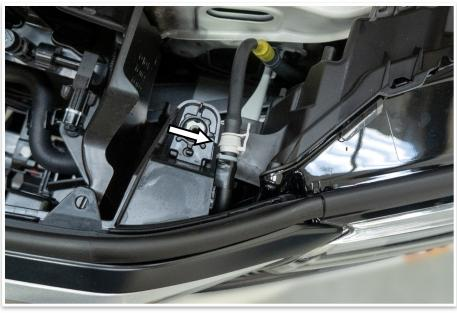
12. Where fitted, disconnect the headlight washer hose at the join shown.
