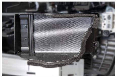
23. Remove both intercooler air guides.
