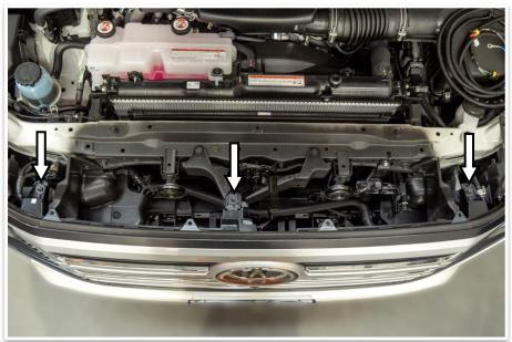
10. Remove the three M6 bolts securing the top of the grille. Retain for reinstallation.
