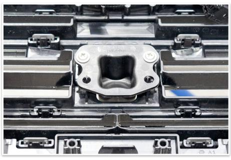
47. Fit the camera blanking plug into the original camera location and fasten using the original screws.
