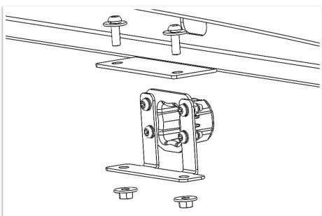
63. Fit camera bracket to the bar using two M6 combo bolts and M6 flange nuts.
