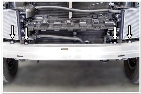
24. With the air guides removed you have access to the top bolts securing the intrusion beam. Remove the four bolts.
