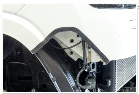
59. Fit the supplied pinch mould to the trimmed edges of the bumper bar and flares.
