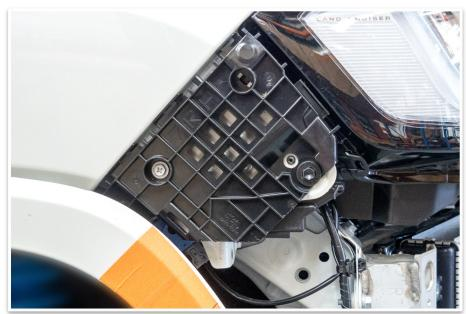
31. After trimming, replace the brackets using the original fasteners.
