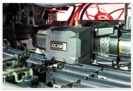
60. Where a winch has been fitted it may be necessary to trim the bottom of the grille to give adequate clearance. This will depend on your winch and control box location.
