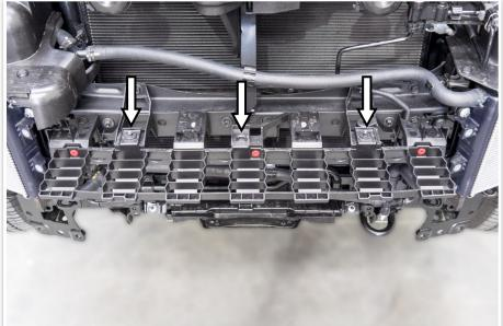
27. There are three bolts securing the bumper bar support. Remove and discard the bumper support.
