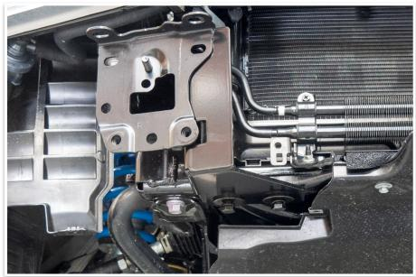
34. Fit the inner chassis support brackets (item # 5 & 6). Secure the lower part of the bracket using the fasteners removed in step 33.
