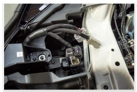
Disconnect the looms, where fitted, for the front camera, parking sensors and fog lights.
