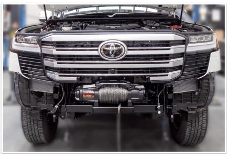
58. Refit the bumper and grille to the vehicle using the original fasteners.
