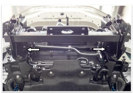
39. On the inside secure with two M12 x 1.75 x 40mm hex bolts, four M12 x 32mm flat washers, two M12 spring washers and two M12 hex nuts. Leave finger tight.
