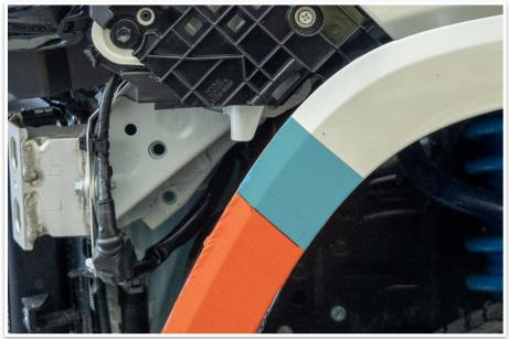
32. Using a grinder, saw or multitool, trim both flares as previously marked.
