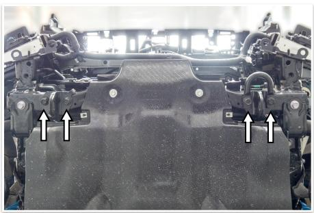
33. Underneath the vehicle, remove the tie downs and tow point. Keep the fasteners.
