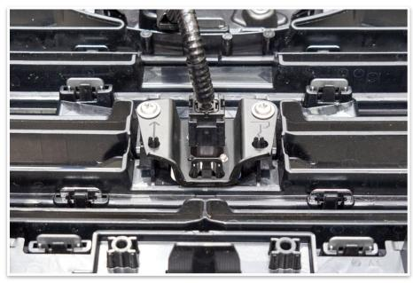
46. If fitted, disconnect and remove the camera.
