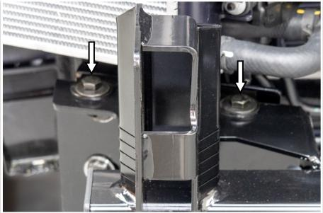
40. Secure the top of the winch mount to the chassis end plate using four M10 x 30mm hex bolts, eight M10 flat washers and four M10 nyloc nuts. Finger tighten only.
