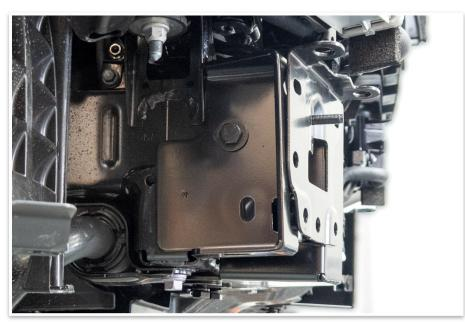
35. Fit the outer chassis support brackets (item # 3 & 4) to the vehicle using two M12 x 110mm hex bolts, two crush tubes (item # 13), four M12 flat washers, two M12 spring washers and two M12 hex nuts. Do not tighten.
