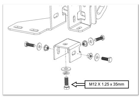
36. Fit the chassis support brackets (item # 7 & 8). These brackets fit to the bottom of the chassis in between the inner and outer chassis brackets. Secure with six M10 x 1.25 x 30mm hex bolts, six M10 flat washers and M10 flange nuts. Secure to the chassis with two M12 x 1.25 x 35mm hex bolts, M12 spring and flat washers.
