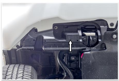
Underneath the bumper bar, remove and discard the fasteners securing the outer cover panels.
