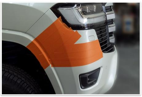
3. Apply masking tape to both sides of the bumper as shown.
