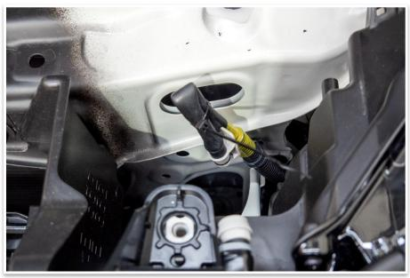
Use a tube clamp or cable tie to stop the washer fluid from leaking.
