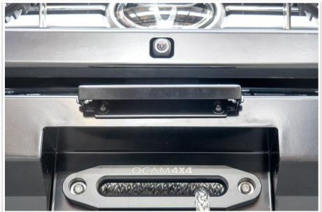
73. If a winch is fitted, fit the number plate bracket (item # 16)to the bar using two M6 combo bolt sets.
