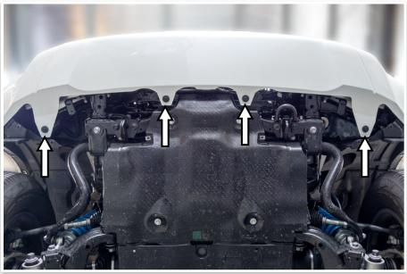
20. Remove and discard the fasteners securing the bottom of the bumper bar.
