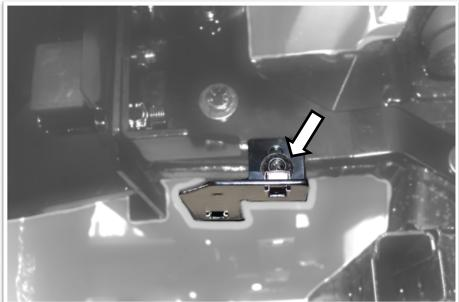
30. Install strengthening brackets with M8 bolt with spring washer, flat washer and nut. Install M6 captive nuts to brackets.
