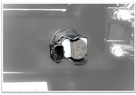
13. Install parking sensors to housing and stick foam pad to sensor.
