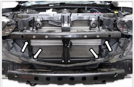
21. Remove 4x retaining clips and remove and discard lower radiator shroud.
