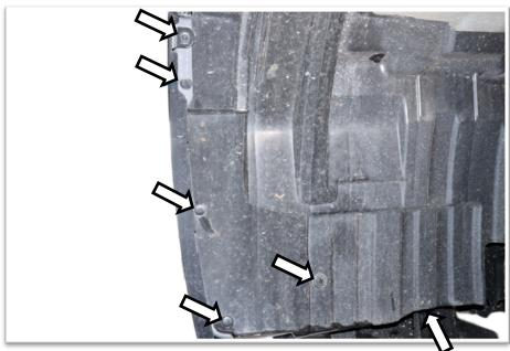
4. Remove 1x screw, 1x nut, and 4x retaining clips to release wheel arch liner from bumper cover.
