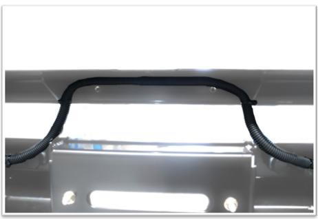
16. Wire vehicle harness to lights in bull bar, secure harness and connect to parking sensors
