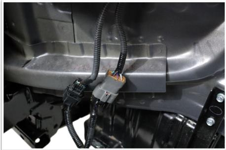
8. Disconnect 2x electrical connectors located below the LH headlight assembly to release the bumper harness vehicle.
