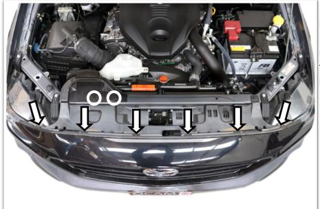
1. Remove 2x retaining clips from intake pipe and remove intake pipe. Remove 6x retaining clips from nose cone, release rubber strip from 2 clips on either side. Pull nose cone forward to remove.
