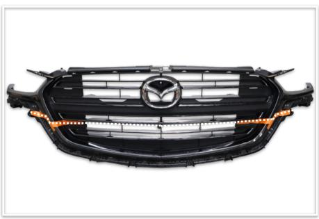
11. The grille will need to be cut to suit the bull bar. Use the image as a guide and follow the shape of the grille to find where cut.
