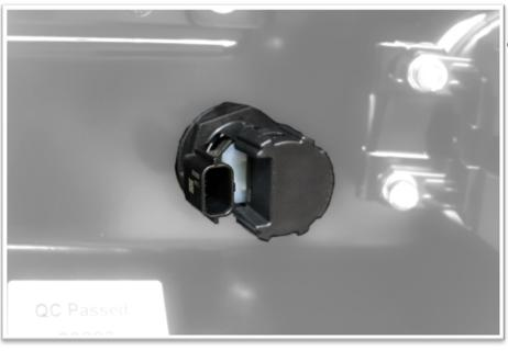
14. Secure sensor in place with rear clip.
