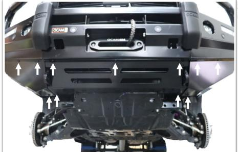
33. Install front and side bash plates using 17x M6 button head screws.
