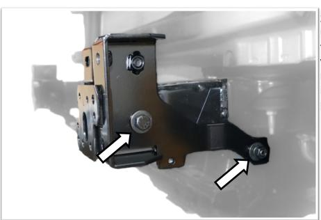
23. Install outer chassis bracket using M10 bolt with spring washer, flat washer and nut for rear. M12 with spring washer, flat washer and nut on front, this will fix through inner chassis bracket and bash plate bracket.
