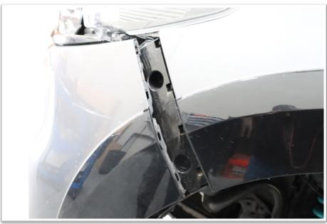
Pull bumper outwards from where it clips into the quarter panel to remove bumper.
