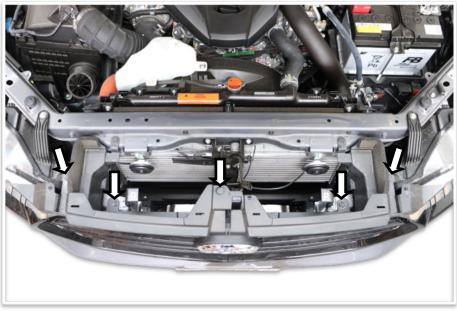
3. Remove 7x retaining clips and 1x screw to release grille. Screw is located in the badge.
