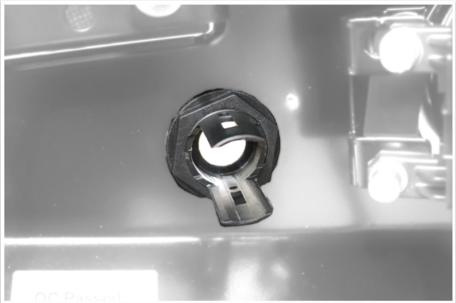
12. Install parking sensor housing to bull bar by inserting into hole and securing with nut.
