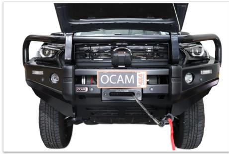
34. Installation is completed, double check all fixings are torqued correctly and all tools are accounted for and packed away.
