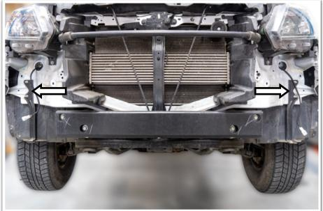
Remove the bumper bar retaining brackets from the vehicle.
