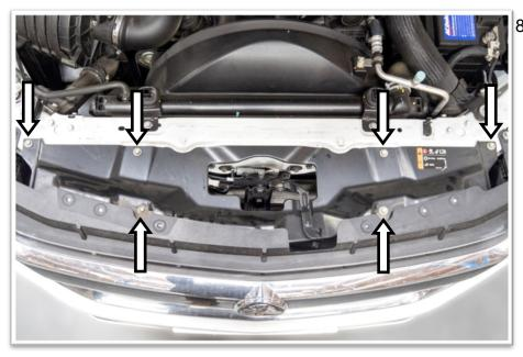
Remove the metal panel from the radiator support panel.
