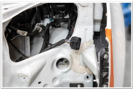
12. Remove the headlights to gain access to the connectors.
