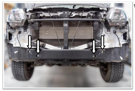
18. Remove the intrusion beam.
