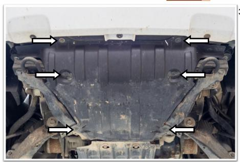
From underneath, remove the plastic stone tray.
