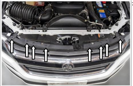
7. Remove the Torx screws that secure the top of the grille. Keep these as they are needed when refitting the grille.
