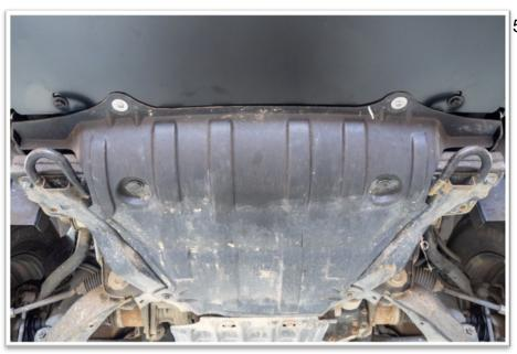
56. Reinstall the plastic stone guard to the vehicle using the original fasteners at the rear and middle. At the front use two M6 dome head bolt sets.
