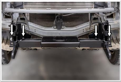
29. Lift the winch mount (item 2) onto the chassis. Secure using the fasteners removed with the intrusion beam.
