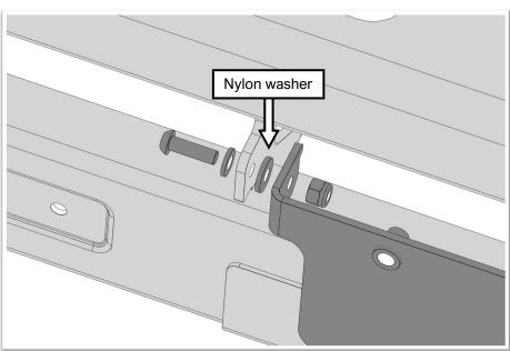
45. Fit the hinged number plate bracket (item 11 to the bar using two M6 x 20mm button head screws, M6 flat washer, M6 nylon washer and M6 nyloc nut.
