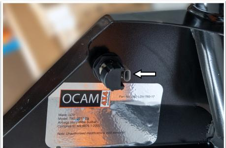
44. Where fitted, install the sensors removed from the bar into the sensor holders, secure with the supplied clamping top section.
