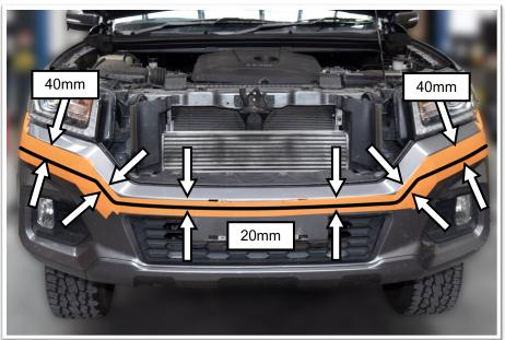
14. From the ends of the template use a marker to connect the both sides as shown below.40mm from the crease under the headlights and 20mm under the crease around the grille opening.
