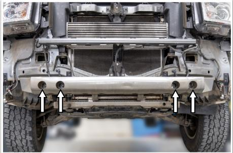
23. Remove the front intrusion beam. Keep the fasteners for installation of the winch mount.
