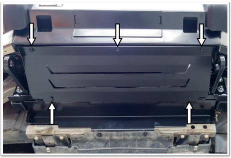
56. Fit the front bash plate (item 7) to the bar using five M6 combo bolts.
