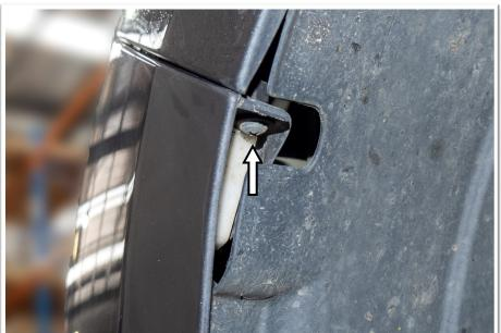
16. Remove the screw from either side of the bumper bar that secures the bumper to the guards. Keep for reinstallation.
