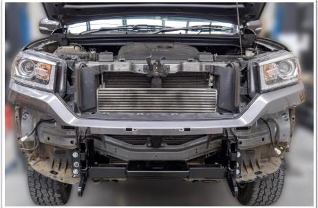
41. Reinstall the trimmed bumper bar, grille and top cover to the vehicle using the original fasteners.
