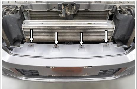
Remove the four screws securing the top of the bumper bar. Keep for reinstallation.
