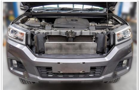
7. Carefully remove the grille from the vehicle.
