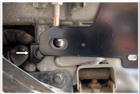
33. At the rear of the outer chassis brackets, insert the chassis spacer (item 13) between the bracket and chassis.
