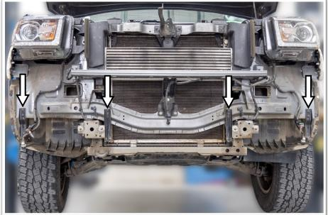
24. Remove the four bumper support brackets.
