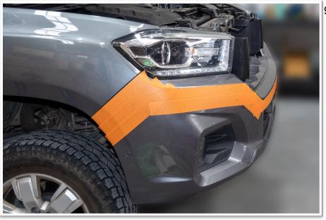
9. Apply masking tape to the sides of the bumper bar as shown.
