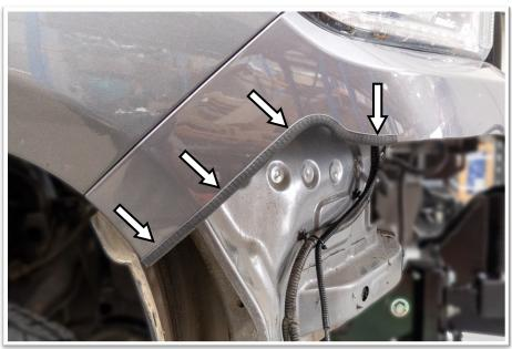
42. Fit the supplied pinch mould to the ends of the bumper bar.
