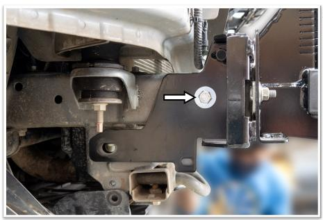
30. Fit the outer support brackets (items 3 & 4) to the chassis using M10 x 90mm hex bolts and flat washers.
