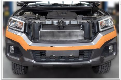
8. Apply masking tape to the front of the bumper bar as shown.
