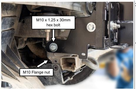
34. Secure the end of the outer chassis brackets using a M10 x 1.25 x 30mm hex bolts, M10 flat washers and M10 flange nuts.
