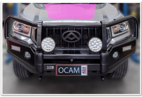
63. Where removed, refit the number plate to the number plate bracket using two M6 combo bolts.
