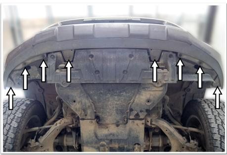
17. Remove the four plastic clips and four screws from the bottom of the bumper bar. These can be discarded as they are no longer needed.
