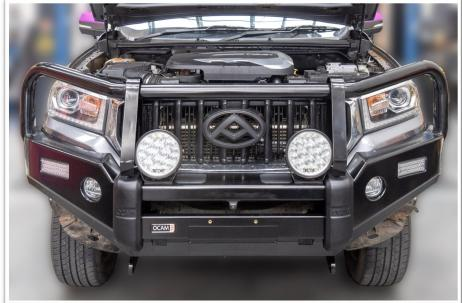
48. Install the bull bar to the vehicle using six M12 x 40mm hex bolts, six M12 spring washers, 12 x M12 flat washers and Six M12 hex nuts.
