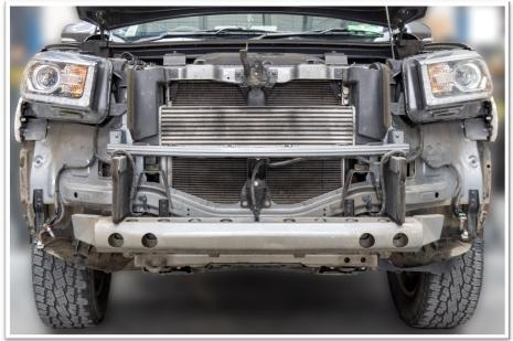
Remove the bumper bar from the vehicle. Place on a stand or protected surface.
