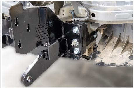
35. Secure the outer chassis brackets to the winch frame using four M10 x 35mm hex bolts, M10 flat and spring washers.
