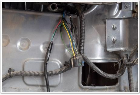
25. Use a LED test light or Multimeter to confirm the vehicles indicator, park and DRL positive wires from the headlight harness.
