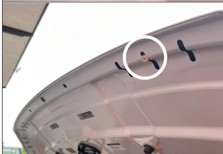
**2. Locate the elongated holes on the underside of the bonnet. Use the middle elongation as pictured and install 1 x small screw grommet. Repeat for the opposite side.**
