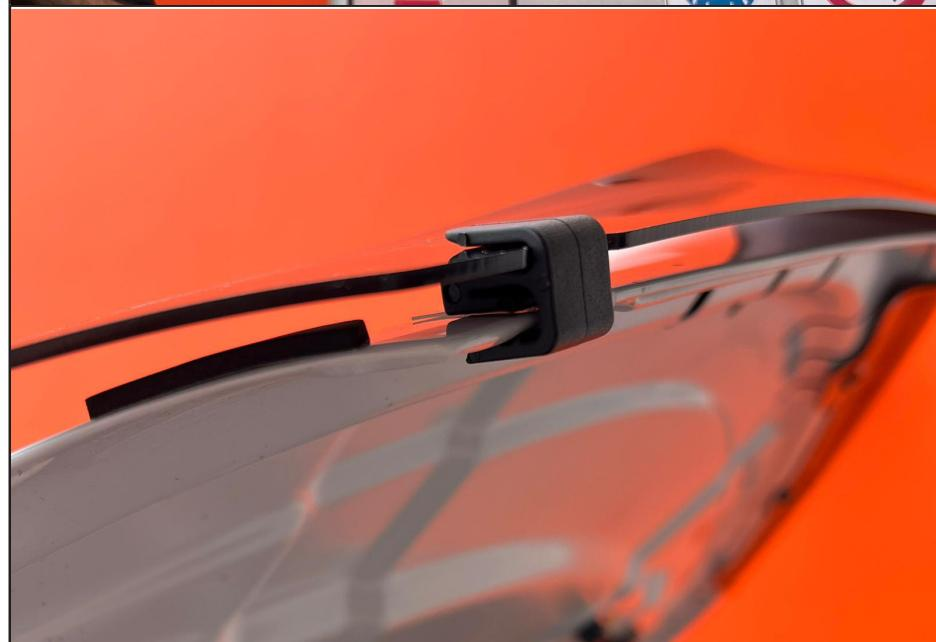
**5. Push hood mounting clip over the abrasive tape and the bonnet protector should be secure.**
