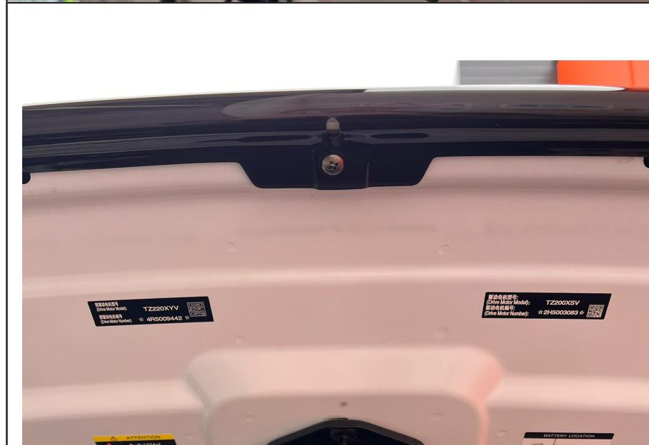
**3. Fit the bonnet protector and fasten the middle tab with 1 x large screw. Then fasten the other 2 mounts with the small screws.**
