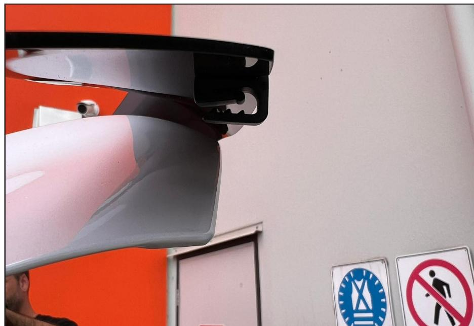
**4. Fit hood mounting clip to bonnet protector. Align and install abrasive tape per to avoid paint being damaged by the clip. Repeat for the other side**
