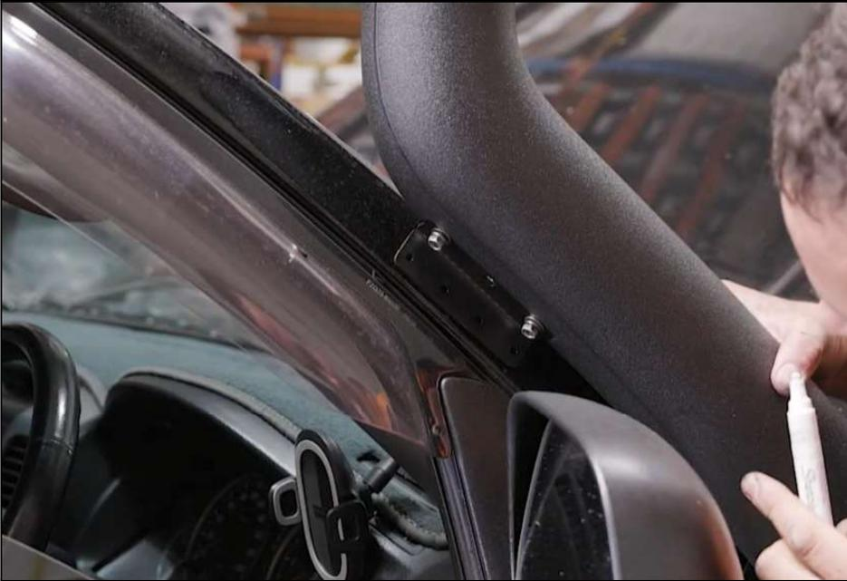
**9. Attach A-pillar mount bracket to snorkel and align snorkel on vehicle. Mark position of mounting holes on A-pillar.**
