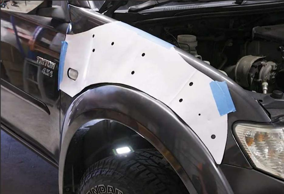
**4. Apply template to quarter panel using masking tape to secure in place. Mark out holes to be drilled and centre punch.**
