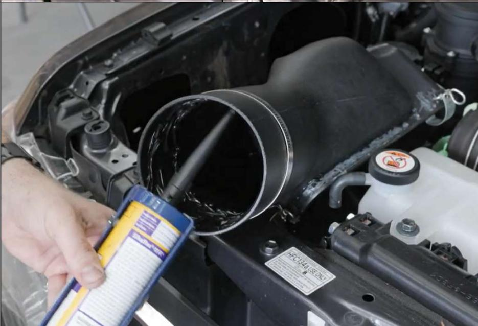
**17. Apply sealant to inner mating surface for airbox duct.**
