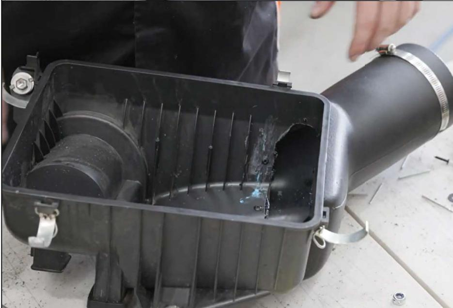
**13. Install airbox attachment, secure with pop rivets supplied.**
