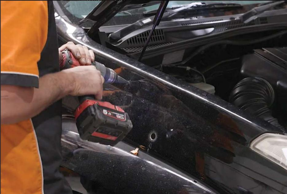
**5. Drill holes as per template. Use debur tool or file to clean off any rough edges or tags.**
