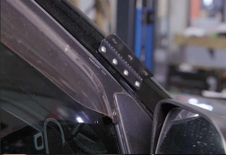
**10. Centre punch and drill holes for A-pillar mounting bracket. Clean up with debur tool and apply touch up paint. Install bracket using supplied hardware.**
