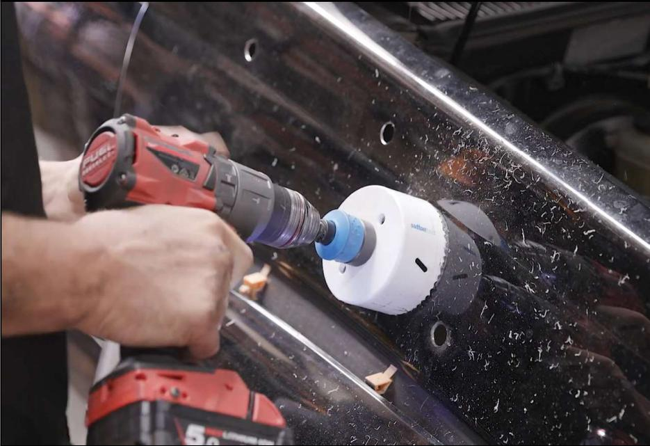
**6. Use hole saw or air hacksaw to cut snorkel duct hole as per template. Use debur tool or file to clean off any rough edges or tags.**
