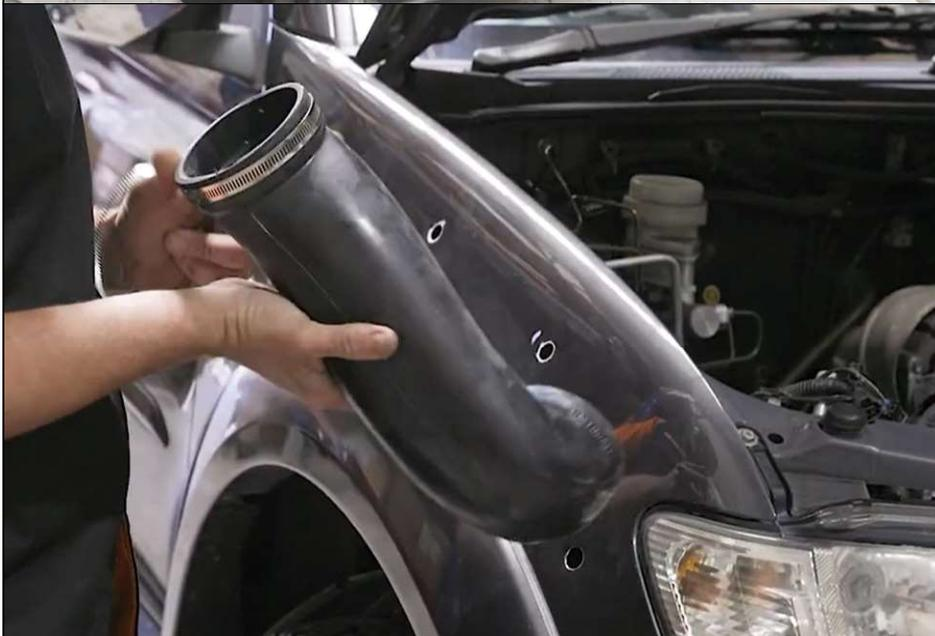
**14. Fit hose clamps to snorkel duct apply sealant to inner mounting surface and position in quarter panel.**
