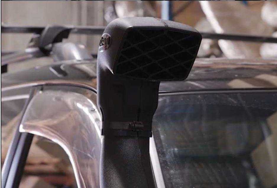
**20. Install snorkel head and secure with clamp.**
