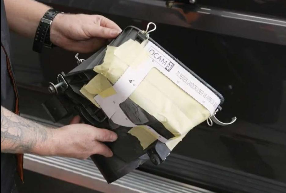
**11. If modification of airbox is required, apply template to airbox and mark cut locations.**
