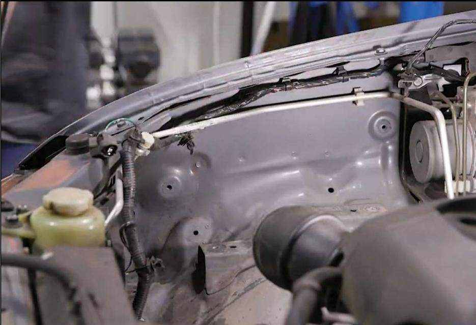
**3. Washer bolts, coolant reservoirs, wiring harnesses, and A/C pipes etc. may need to be relocated or temporarily removed/ mover asside for access. (Snorkel kit will include parts for relocations required).**
