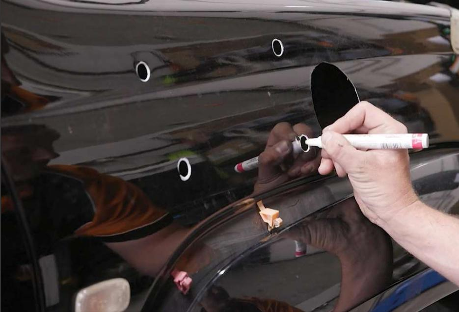
**7. Apply touch up paint to holes to prevent corrosion.**
