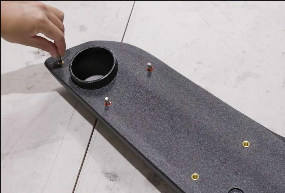
**8. Insert mounting studs into threads in snorkel body where required.**
