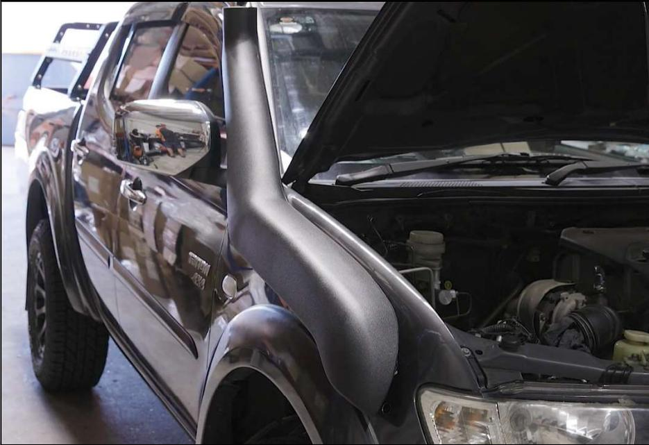
**15. Install snorkel to quarter panel and secure duct to snorkel flange.**
