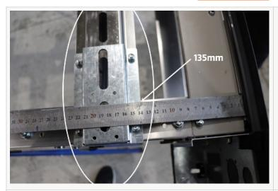
At the rear of the drawer module, ensure the mounting rail begins 135 mm from the rear-most edge of the module.
