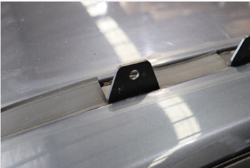
Installed roof brackets (Side view)
