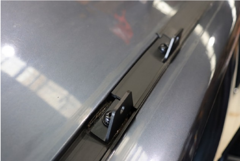
Installed roof brackets
