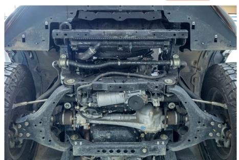
If necessary, clean underneath before fitting the new bash plates.
