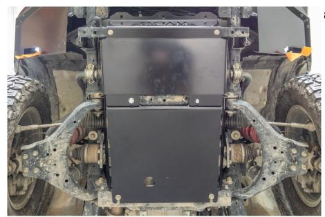
8. Align both bash plates and tighten the fasteners to the correct torque.
