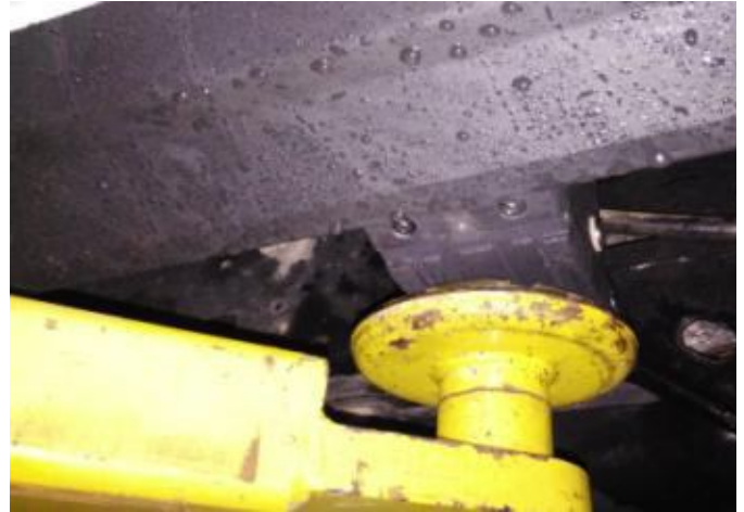
DEMO: CORRECT HOIST LIFTING
