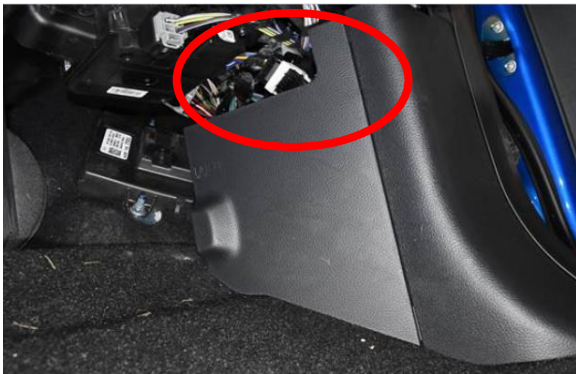
3) Locate wiring at right upper position
