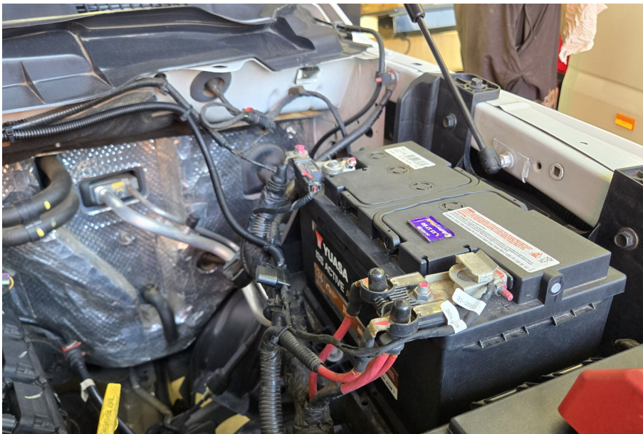
2. Connecting positive pole with battery
