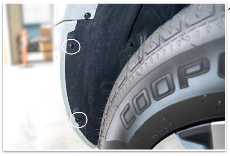
Remove the two screws (both sides) that secure the guard liner to the bumper bar.
