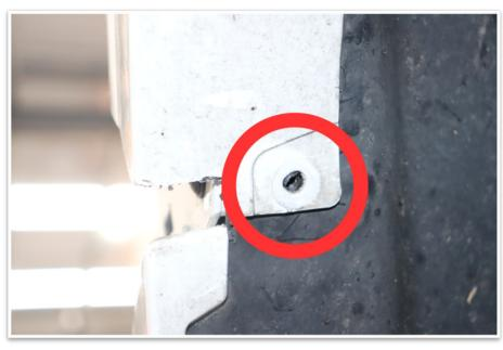
When trimming flares, be careful not to remove mounting hole on inside lip of flare.
