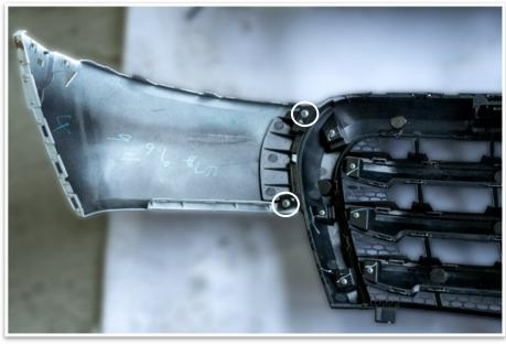
50. Reattach the outer bumper section to grille using the original fasteners.
