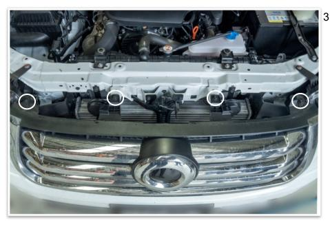
3. Remove the four hex bolts that secure the top of the grille. Retain the bolts for reinstallation.
