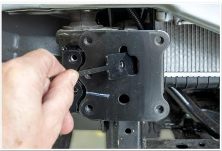
27. Place the short M12 nut plates (item # 18) into the hole in the front of the chassis end plate.
