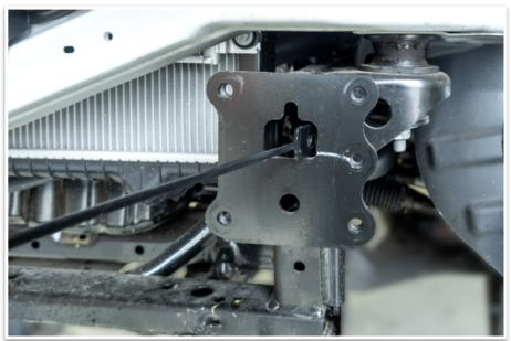
25. Insert the long M12 nut plates (item # 17) into the hole in the front of the chassis end plate.
