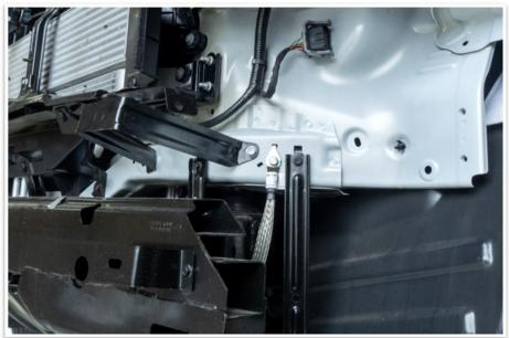
18. Remove the brackets, eight in total, that supported the bumper bar.
