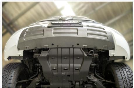
From underneath, remove the fasteners securing the bumper bar.
