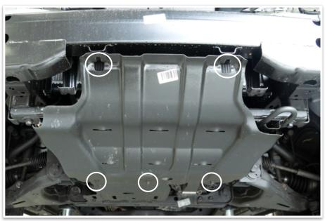
17. Remove the front stone tray from the vehicle. Set aside for refitment. Retain the fasteners.
