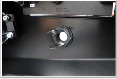
56. Insert sensor seat and secure with nut.
