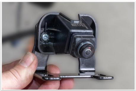
61. Using two M5 screws, M5 flat washer and M5 nyloc nut, attach the camera to the camera bracket (item # 16) as shown.
