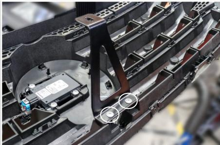
53. Fit the grille bracket (item # 15) to the grille using the screws that secured the camera.
