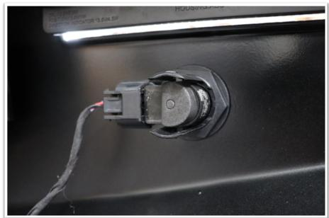
57. Install parking sensors to sensor seat and apply foam pad to back of sensors.
