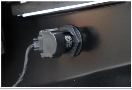
60. Secure sensors in place by clipping on rear cap.
