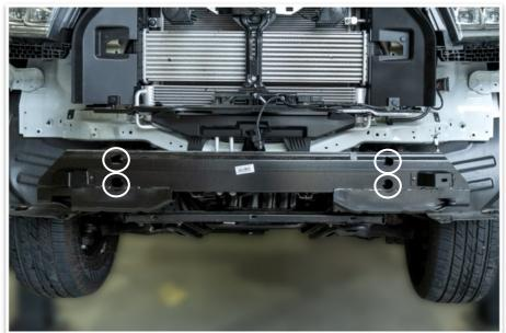
21. Remove the front intrusion beam.
