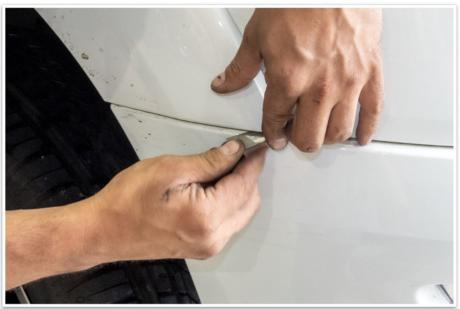
6. Using a sharp knife, trim the tab between the flare and bumper that locates the flare to the bumper bar.
