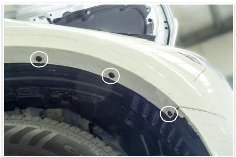
Remove the three screws (both sides) that secure the flare to the guard liner. Keep the top two screws.
