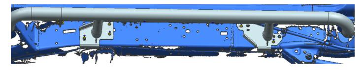
4. Fasten the side step with flat washers, spring washers and nuts provided.
