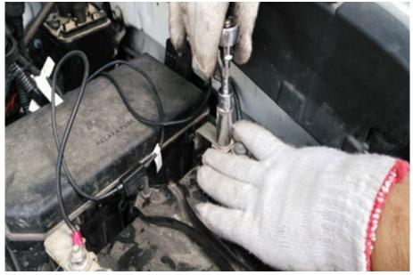
2. Connect power wire to battery: red one with fuse is positive.
