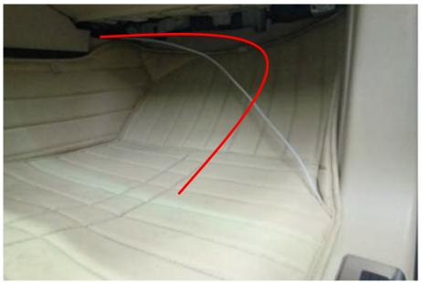
7. Right motor wire and OBD line from this position to drive site
