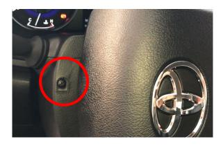
1. Start engine, disassemble 3 screws under steering. **Then shut down engine.** Take off the plastic cover under steering
