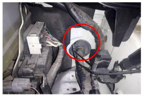
4. The wiring from this position to co-drive cabin
