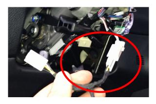
3. Plug with our connector then insert it back to original position. Recover all parts back to vehicle
