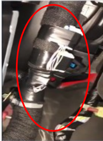
Connector is covered by tape with wiring. Carefully cut the tape to release the connector/harness.
