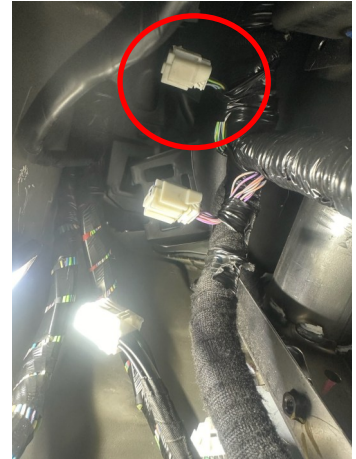
Remove the original connector and insert the supplied adapter harness to the connector shown above. Then piggy-back (re-install) the original connector.
